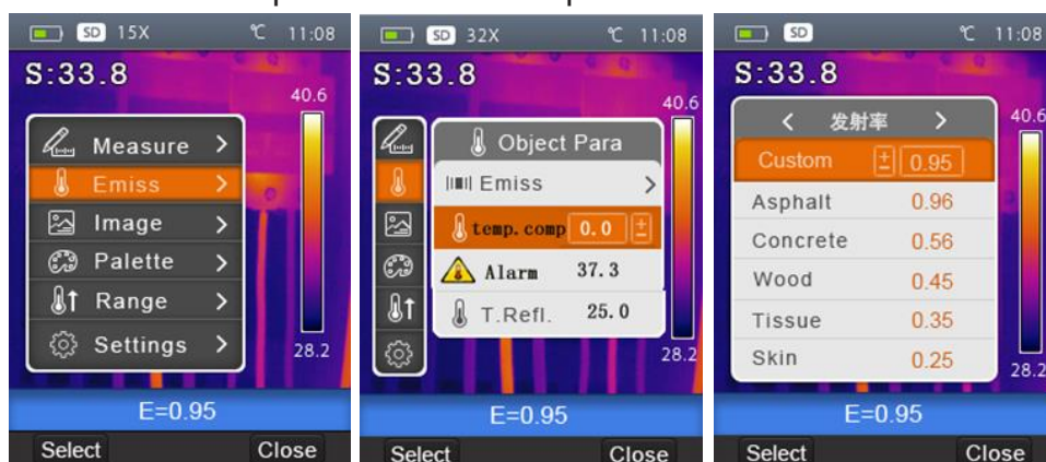
Figure 4: Menus for setting the emissivity, temperature compensation, alarm and reflected temperature.
